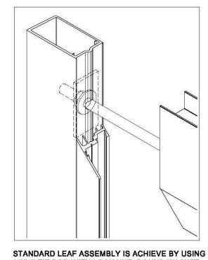
STANDARD LEAF ASSEMBLY IS ACHIEVE BY USING 3/8" Ø TIE ROD WITH LOCK NUT, ROUND WASHER AND 3/16" THK. RECTANGULAR ALUMINUM PLATE SUPPORT AT EACH CORNER OF THE LEAF.
